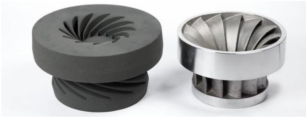
Figure 38: Sandcasting pattern and casting, © Voxeljet
