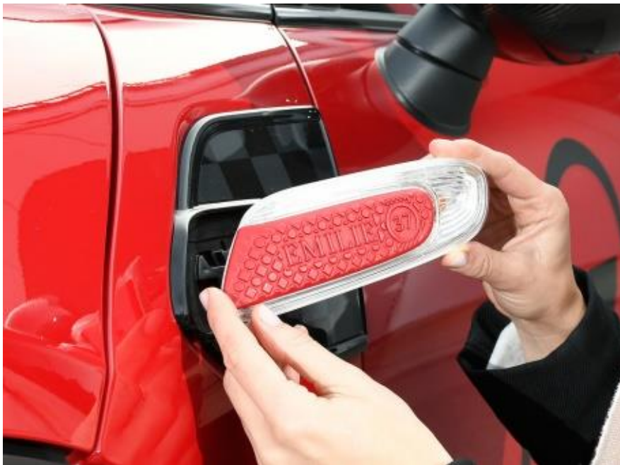
Figure 33: Personalised Mini headlight components, © BMW
